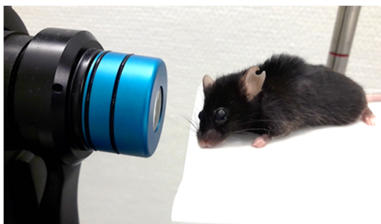
Figure 2. FLIO with mice. (A) Mouse in front of the FLIO device. Because of the short eye of the mouse a 25 D lens (blue) was positioned in front of the FLIO camera. (B) FLIO image and the grid for analysis. In FLIO, infrared reflection image ( left ) and the pseudo-colored FLT images ( right ) are provided. The FLIO data was analyzed by the FLIO Reader software, which uses an Early Treatment Diabetic Retinopathy Study grid consisting of a central region (C), inner ring (IR) and outer ring (OR). In this study, the optic nerve head was placed in (C).
