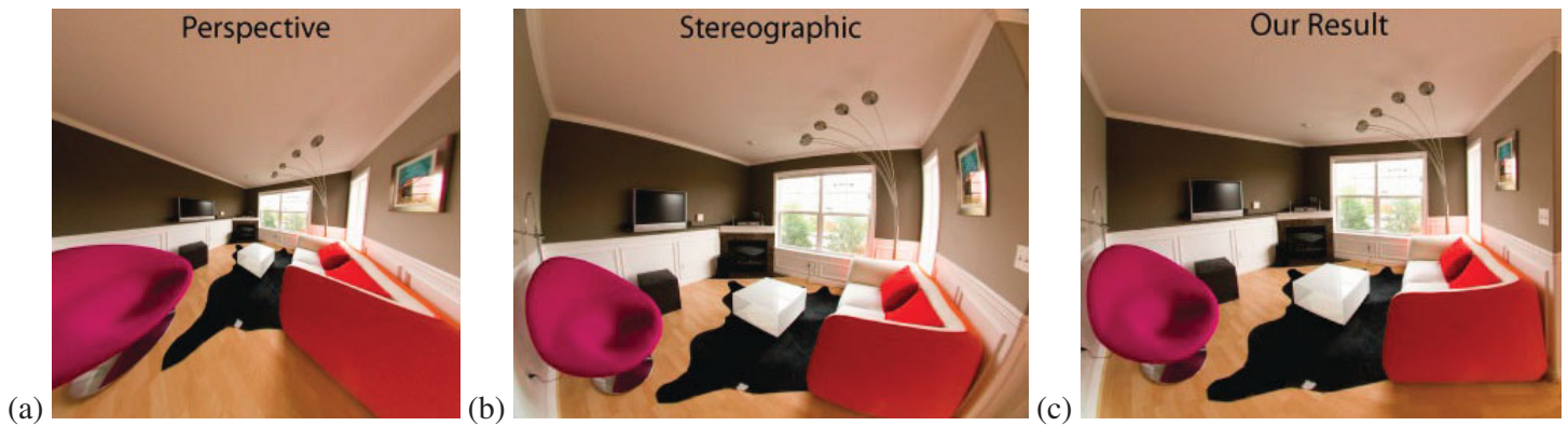
Figure 21. Content-aware projection of wide-angle photography, from Carroll et al. (2009). (a) An input wide-angle linear perspective photograph. (b) A stereographic projection computed from the input photo, which creates new distortions. (c) A content-aware projection computed from the input photo, by warping the input photo, in a way that preserves straight lines and other objects, while allowing textureless regions to warp.
